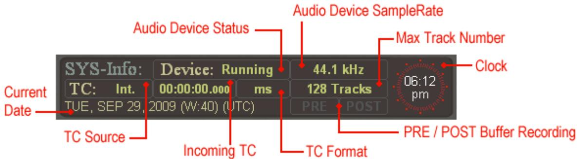
The incoming TC is shown in its original native format. The Format is blinking when chasing if it does not fit the Timecode format of the project (see Transport Option Dialog Box). The audio device sampling rate is also blinking when it does not fit the one from the project.
